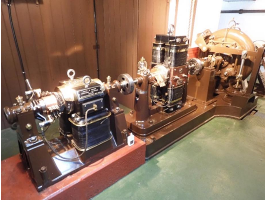
Figure 4.2 The Cragside turbine with both generators on the turbine output shaft (Photograph: Author, 2023).
